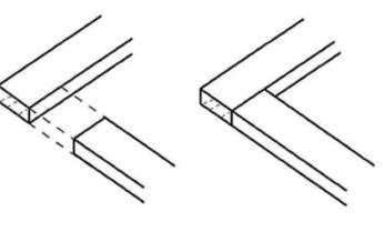
• Mitre join: Generally the most aesthetically pleasing of joints as it hides the endgrain of
